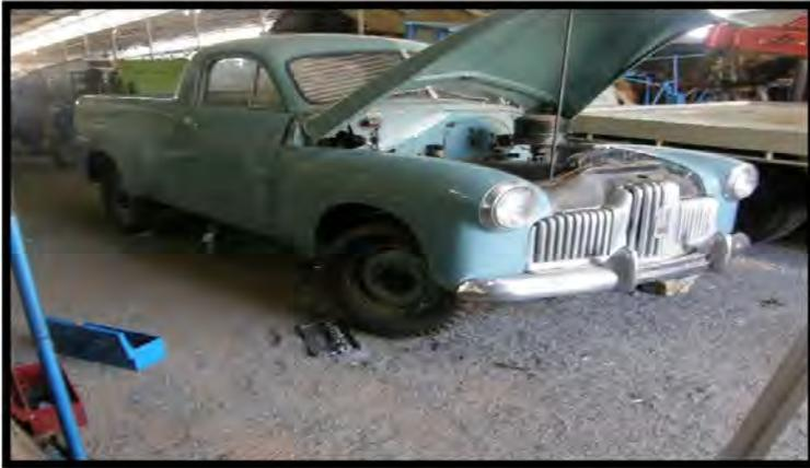
New member Tim experimented with sealing the very dusty floor (when it is not wet!), while Gerry & Eric started to remove the Brake Master Cylinder from the FX Holden Ute, the piston is stuck in the cylinder, so she has no brakes----yet.
