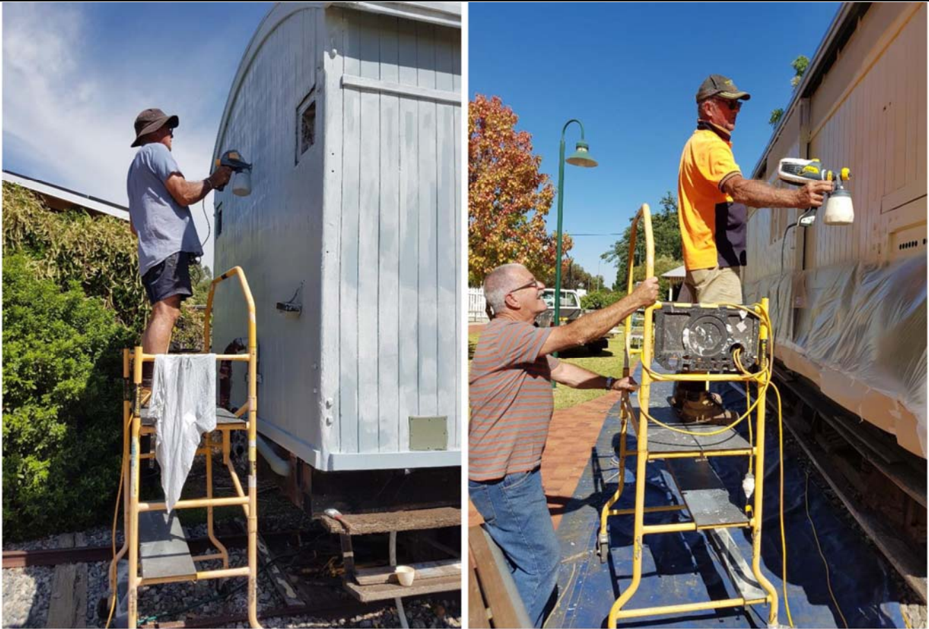
Haydn painting the second undercoat; And AiR Diane Clark's husband Don helping Haydn paint the cream coloured top coat
