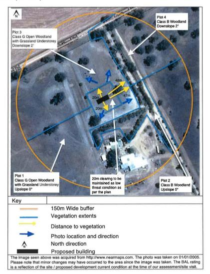
Note: The 150m radius depicted on the site plan is used to identify any classifiable vegetation from the centroid of the proposed building envelope. Any vegetation greater than 100m from the proposed building envelope is excluded from classification as per AS-3959.
